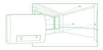
Do Not: Place the sensor in any of the following areas: directly on a window; in a stairwell; near an air vent; in a room smaller than 100 square feet; in rooms with excessive white noise (i.e. fans or other persistent appliance); or in high-humidity areas.
